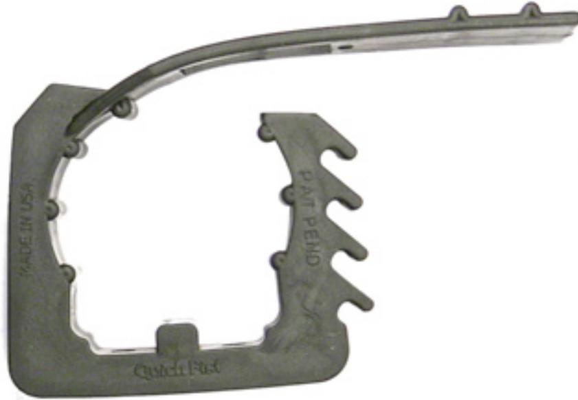
1. Mount with two M6 (1/4") fine thread screws or bolts and washers (under the bolt or screwhead). Do not over-tighten, as the rubber just spreads.
